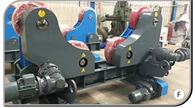
Example : 4WD-4Wheel Driven with Gear Transmission
