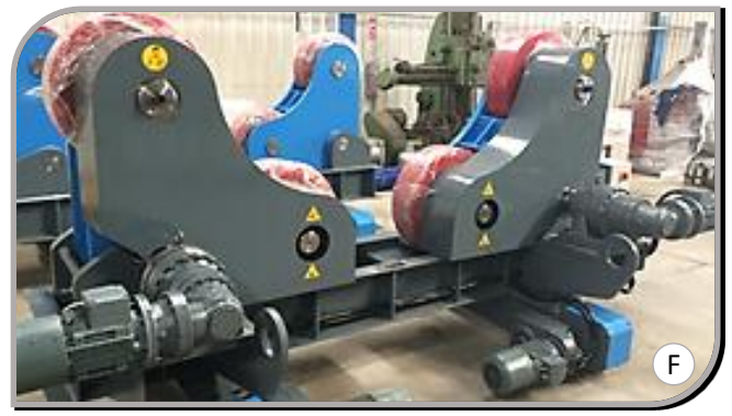
Example : 4WD-4Wheel Driven with Gear Transmission
