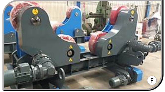
Example : 4WD-4Wheel Driven with Gear Transmission
